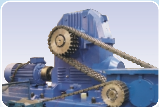
TW Series wormgear units used 14" to 28" centre distance, AC motor, brake coupling and brake with final chain drive. Unit shown being load tested at Renold Gears.
