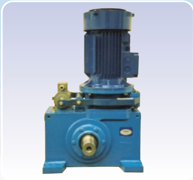
Special wormgear unit manufactured with 3 sizes, using 4", 6" and 8" centre distance wormgears. Unit supplied with vertical AC motor, brake coupling and calliper brake between motor and gear unit.
