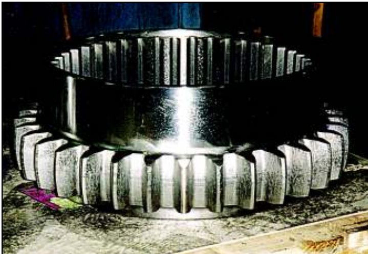
▲ Advanced load-sharing tooth design
