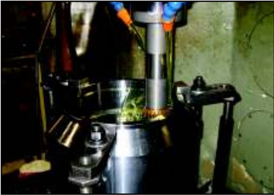
▲ Gear shaping machine
